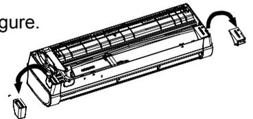
2. Remove 2 gaskets under the cross-flow fan (MVAW018/24MV2AA).
