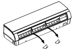
3. Clean the burr on the surface of fracture to avoid the power wire from being scratched after removing the virtual opening of the outgoing line slot on the case by hands in indoor power-on process.
