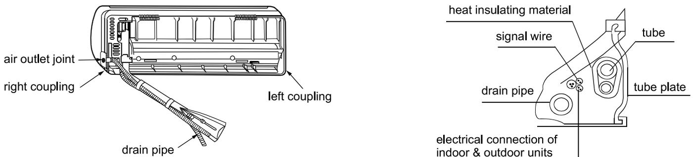
(4) Lead the connection tubing (liquid pipe and gas pipe) through the hole into the wall, or connect piping and wiring of indoor unit (check the number of wiring terminals of indoor and outdoor units and connect terminals with the same number and color), and then put the connection tubing and the connecting line through from the inside wall for the connection with outdoor unit.
