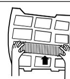
4. Attach the standard air filter (Necessary installation)
