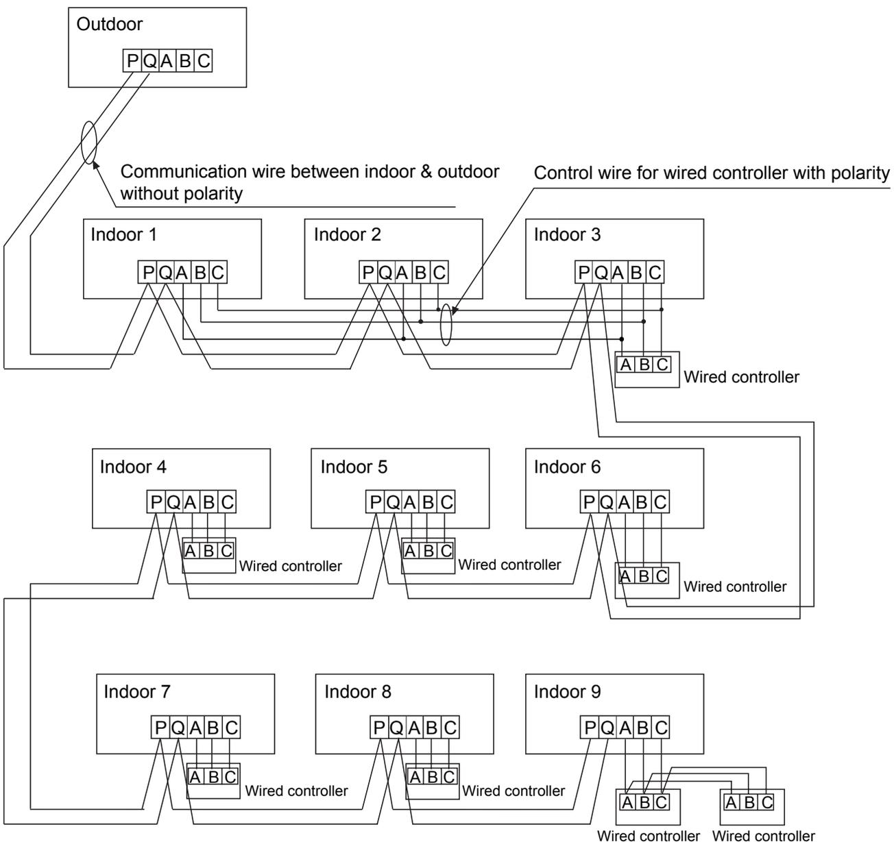
Outdoor units are of parallel connection via three lines with polarity. The main unit, central control and all indoor units are of parallel connection via two lines without polarity.
